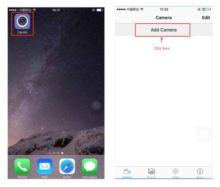
2, There are 3 ways to add IP camera on CamHi: .①Scan camera QR code, ②Search camera from LAN, ③Manual add by camera UID number
